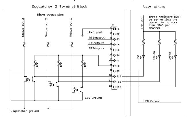
If the RemoteLEDs option is set to TRUE in the configuration file, these LEDs will blink on at the same time as the internal LEDs. If you are reading the voltage at these points you may omit the LED and only use a pullup resistor. Please note that the sigals will be opposite those of the LEDs, when the green LED is off you will read a high voltage on pin 12.
