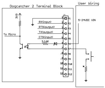
If you wish to use more than 24VDC, Please add a resistor in the circuit to limit the total current to 10mA. The ground connection MUST be referenced to the VIN to this part of the circuit. Design for 1.7V total diode drop.
